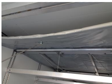
Pull out the partition wall with the rod to the rear until the dividing wall can be gripped by hand.
