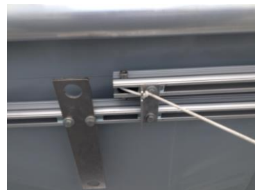
Attach the knot of the release cord to the provided holder
