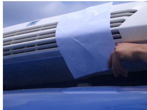
Blade is sucked in - correct polarity
