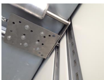
To fix the partition loosen the unlocking cord and make sure that the bolts snap into the side of the loading beam rail.
