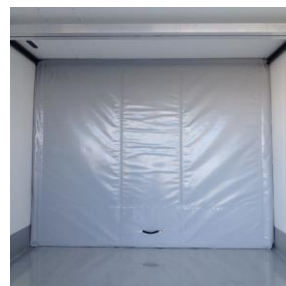
Put the partition wall in vertical position
