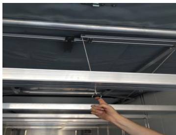
Unlock the locking pin by pulling the cord
