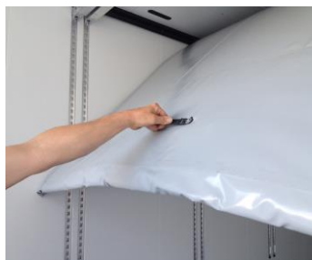
Pull out the partition wall by hand as far as it will go until the partition wall folds down automatically.
